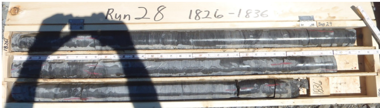
Figure B-32. Run 28: 1,826–1,836 Feet Below Ground Surface. Salina Group-Salina G/Camillus Formation.
