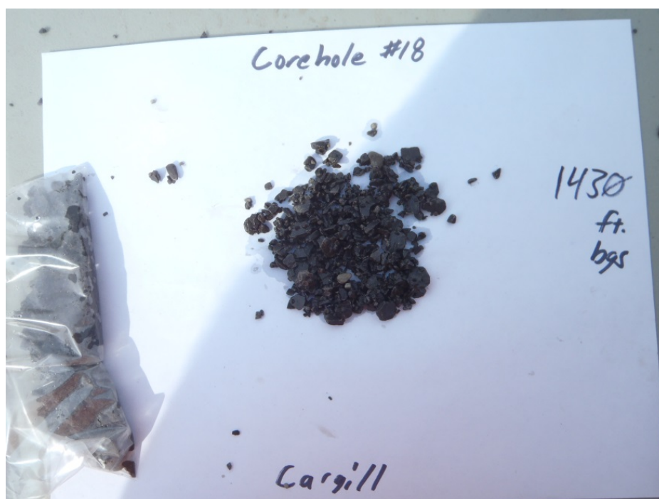
Figure A-74. Corehole #18: 1,430 Feet Below Ground Surface. Hamilton Group: Marcellus Shale Formation–Union Springs Member.
