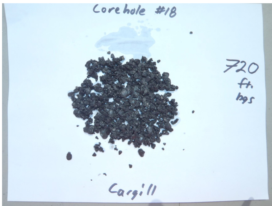
Figure A-37. Corehole #18: 720 Feet Below Ground Surface. Hamilton Group: Ludlowville Shale Formation–Otisco Member.
