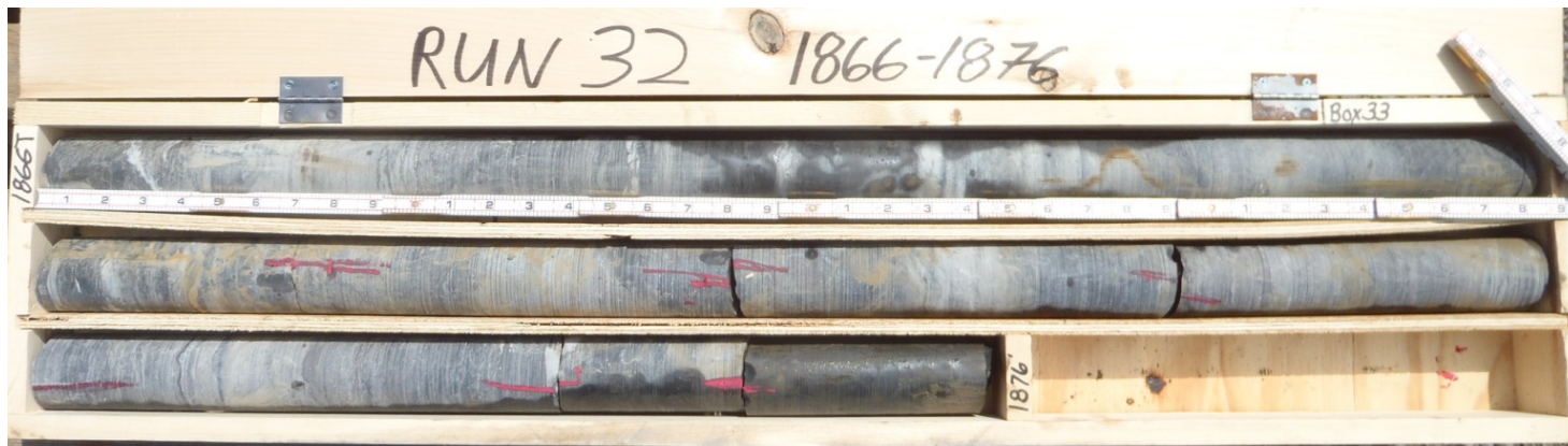
Figure B-36. Run 32: 1,866–1,876 Feet Below Ground Surface. Salina Group- Salina G/Camillus Formation.
