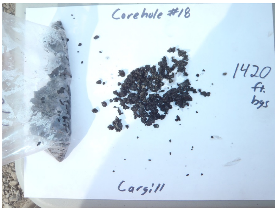
Figure A-73. Corehole #18: 1,420 Feet Below Ground Surface. Hamilton Group: Marcellus Shale Formation–Union Springs Member.
