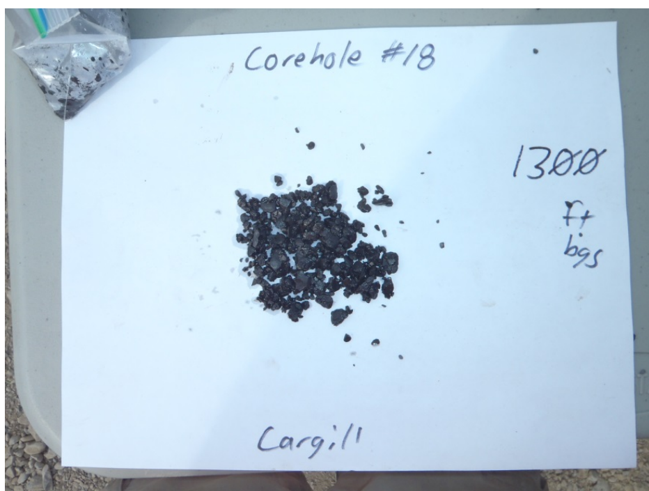
Figure A-66. Corehole #18: 1,300 Feet Below Ground Surface. Hamilton Group: Marcellus Shale Formation-Oatka Creek Member.
