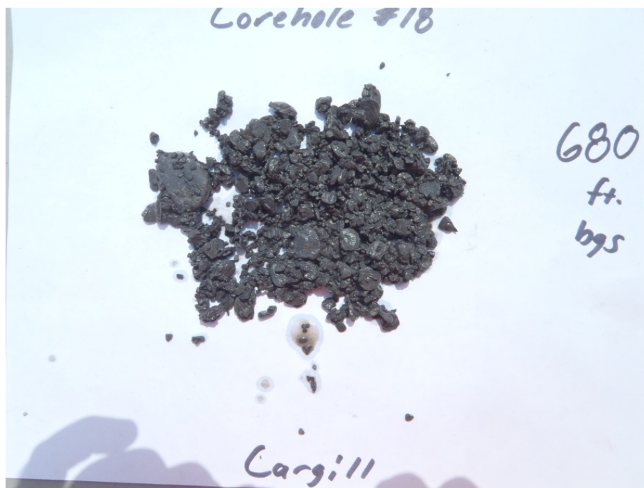
Figure A-35. Corehole #18: 680 Feet Below Ground Surface. Hamilton Group: Ludlowville Shale Formation–Otisco Member.
