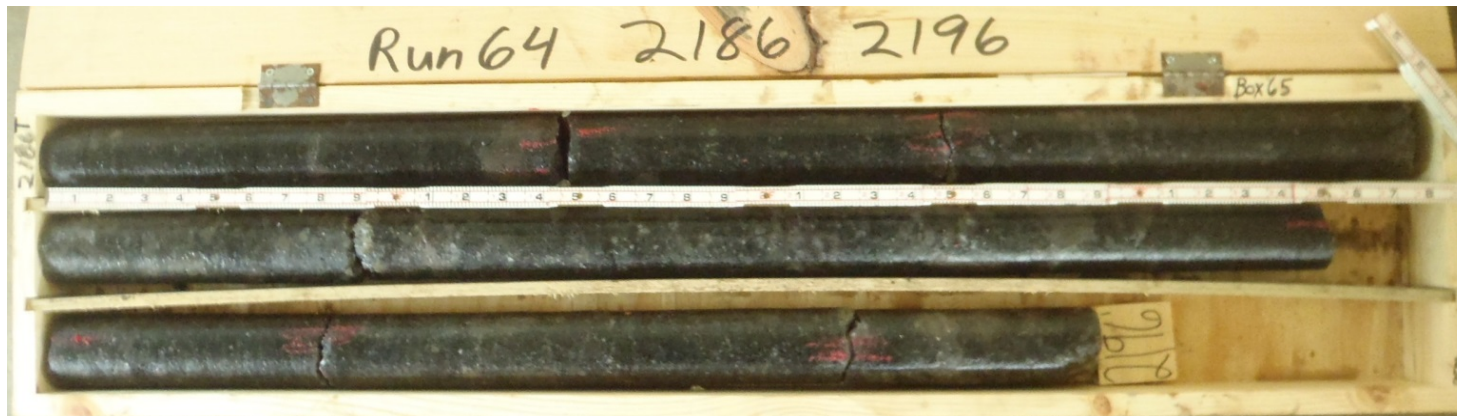
Figure B-75. Run 64: 2,186–2,196 Feet Below Ground Surface. Salina Group: Syracuse Formation–Salina F1/4A Salt.
