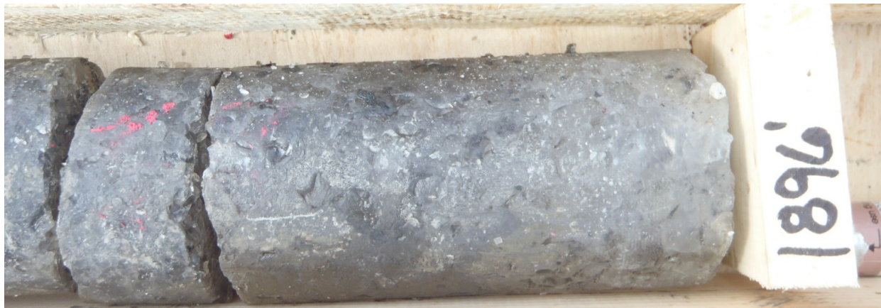
Figure B-40. 1,896 Feet Below Ground Surface. Close-up of Salina F4- #1 Salt.
