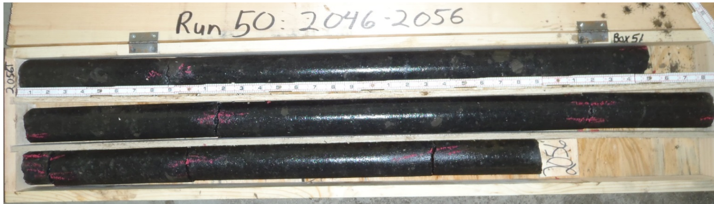
Figure B-61. Run 50: 2,046–2,056 Feet Below Ground Surface. Salina Group: Syracuse Formation–Salina F2/#3Salt.
