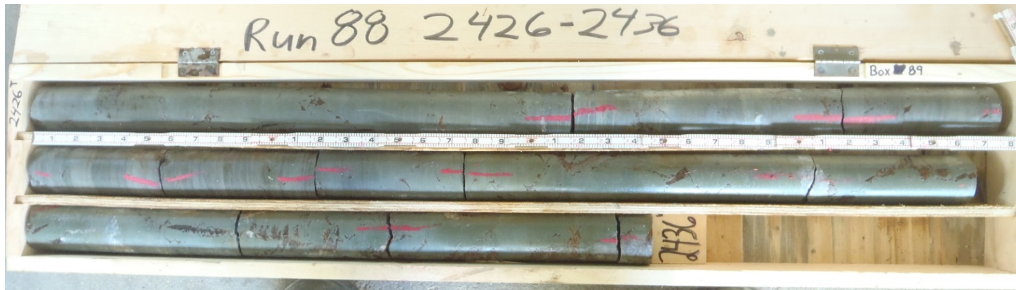
Figure B-101. Run 88: 2,426–2,436 Feet Below Ground Surface. Salina Group: Syracuse Formation–Salina C/Vernon Shale.
