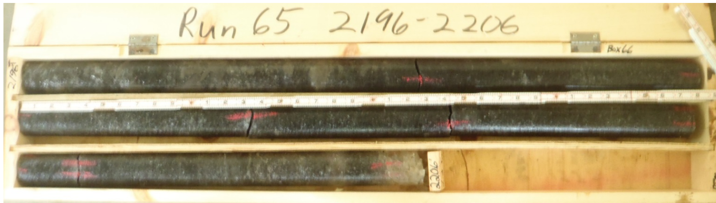
Figure B-76. Run 65: 2,196–2,206 Feet Below Ground Surface. Salina Group: Syracuse Formation–Salina F1/4A Salt.
