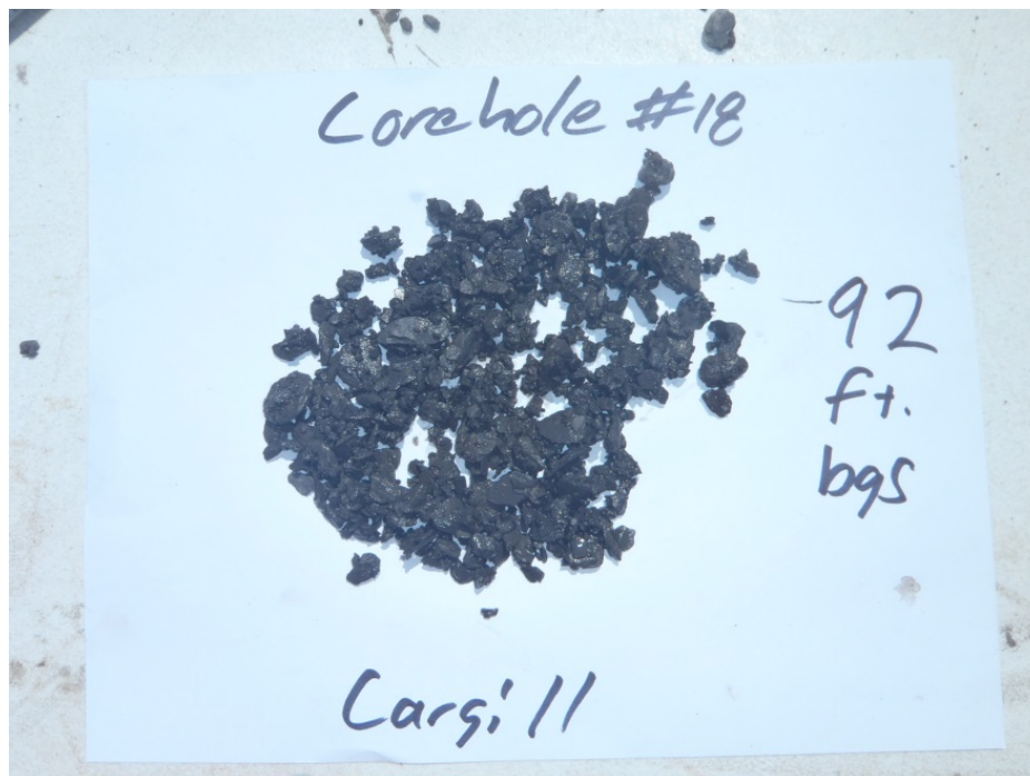
Figure A-5. Corehole #18: 92 Feet Below Ground Surface. Genesee Shale Formation–Sherburne Member.
