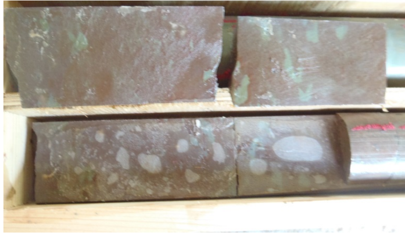
Figure B-107. Brine Bubbles Under the Salt Sheet in the Vertical Fracture at 2,484 Feet Below Ground Surface. Salina Group: Syracuse Formation–Salina C/Vernon Shale.
