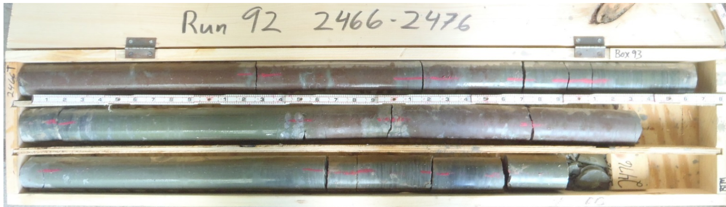
Figure B-105. Run 92: 2,466–2,476 Feet Below Ground Surface. Salina Group: Syracuse Formation–Salina C/Vernon Shale.
