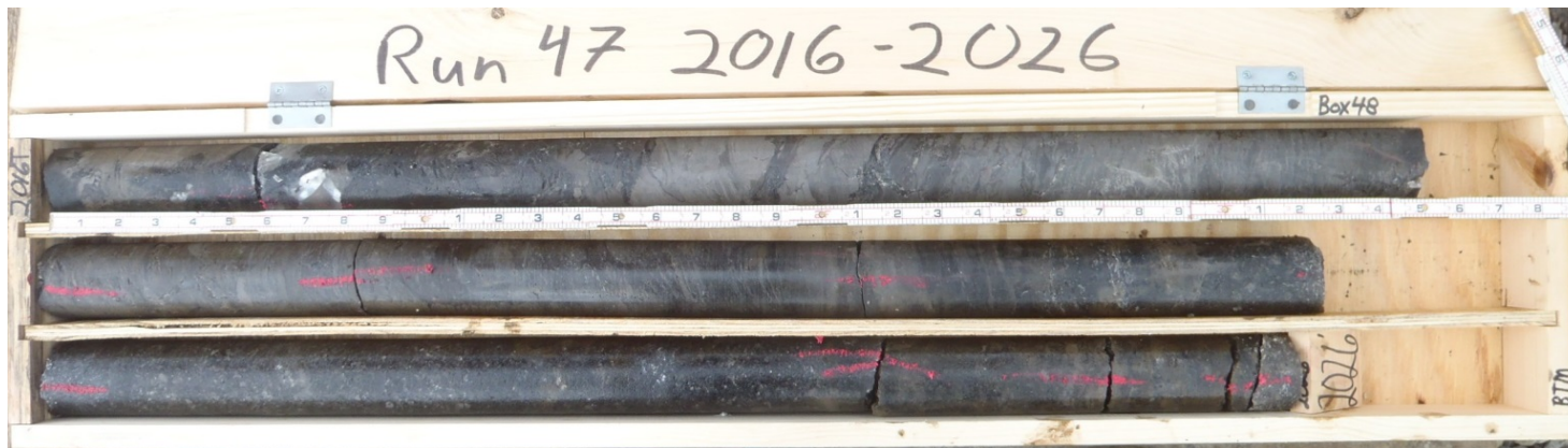
Figure B-56. Run 47: 2,016–2,026 Feet Below Ground Surface. Salina Group: Syracuse Formation–Salina F3–Salina F2/#3 Salt Contact.
