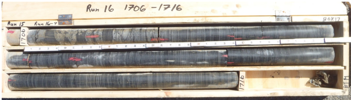
Figure B-20. Run 16: 1,705.8–1,716 Feet Below Ground Surface. Helderberg Group: Bertie Formation–Forge Hollow Member.
