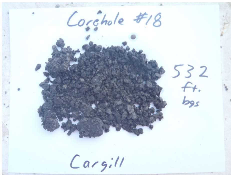
Figure A-27. Corehole #18: 532 Feet Below Ground Surface. Hamilton Group: Ludlowville Shale Formation–Spafford Member.
