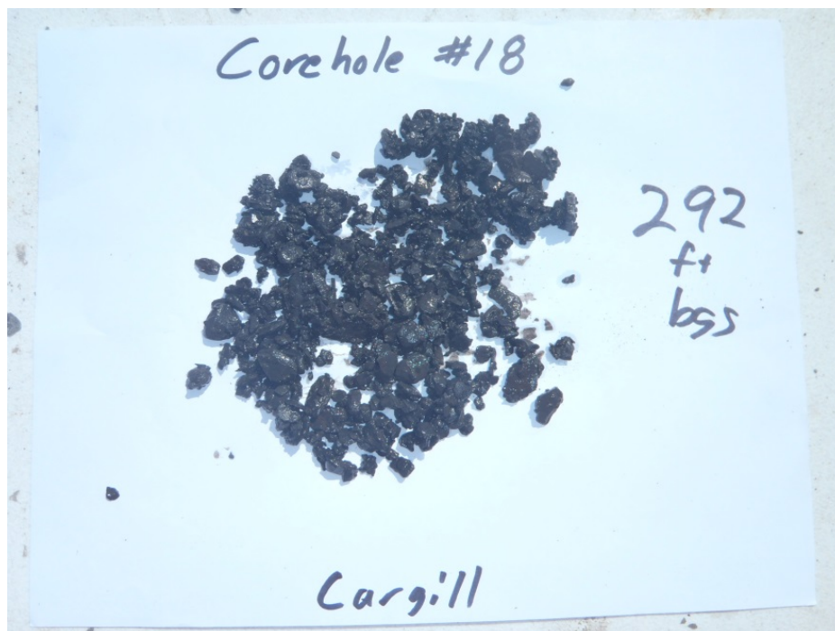
Figure A-15. Corehole #18: 292 Feet Below Ground Surface. Genesee Shale Formation–Geneseo Shale Member.
