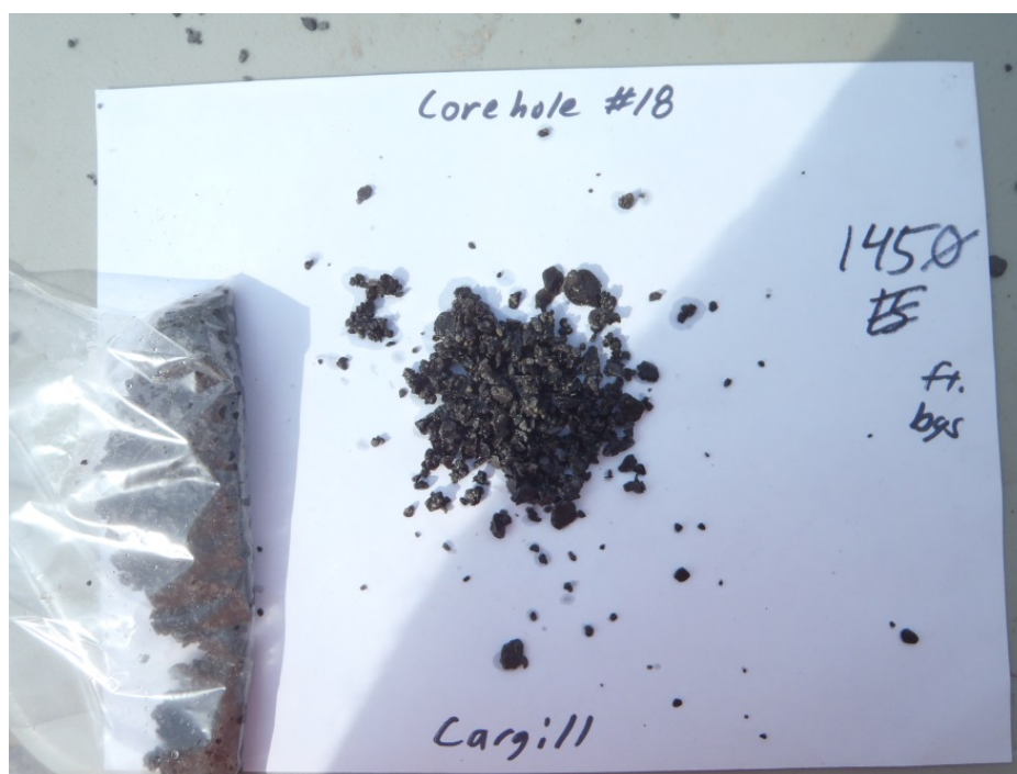
Figure A-76. Corehole #18: 1,450 Feet Below Ground Surface. Onondaga Limestone Formation–Seneca Member.
