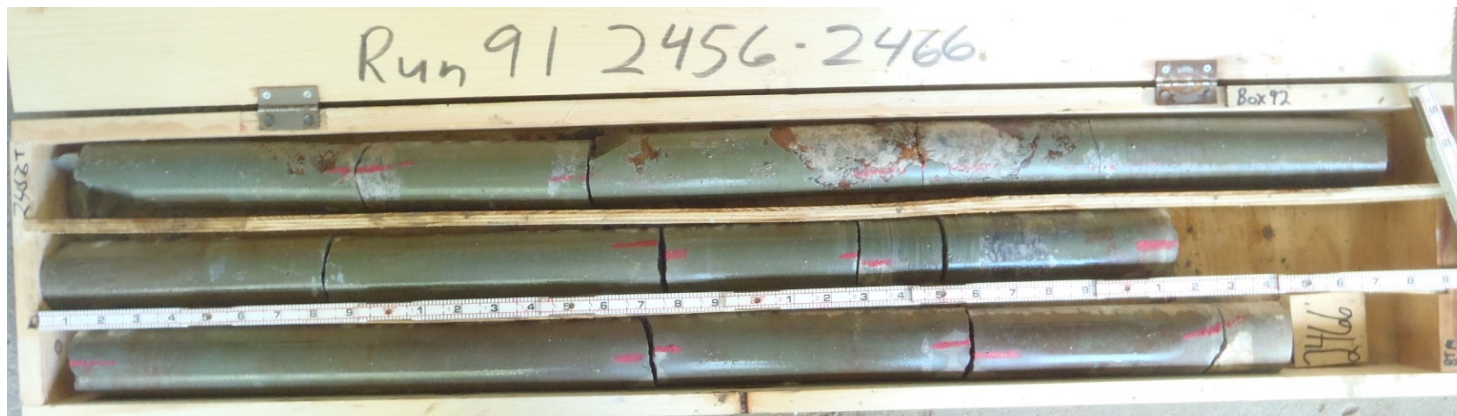
Figure B-104. Run 91: 2,456–2,466 Feet Below Ground Surface. Salina Group: Syracuse Formation–Salina C/Vernon Shale.
