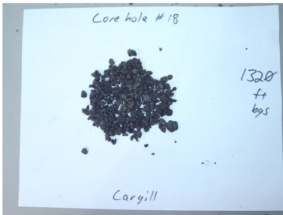
Figure A-67. Corehole #18: 1,320 Feet Below Ground Surface. Hamilton Group: Marcellus Shale Formation–Oatka Creek Member.
