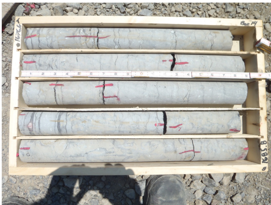
Figure B-16. 1,676.6–1,685.8 Feet Below Ground Surface. Helderberg Group: Cobleskill Formation–“Akron Facies.”
