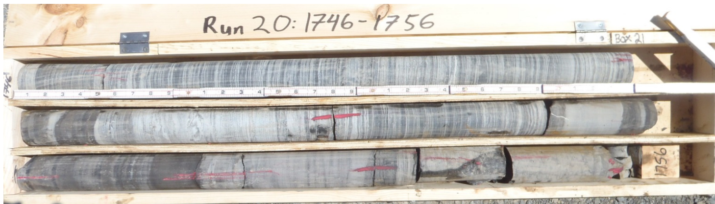
Figure B-24. Run 20: 1,746–1,756 Feet Below Ground Surface. Bertie Formation Helderberg Group: Bertie Formation–Forge Hollow Member.
