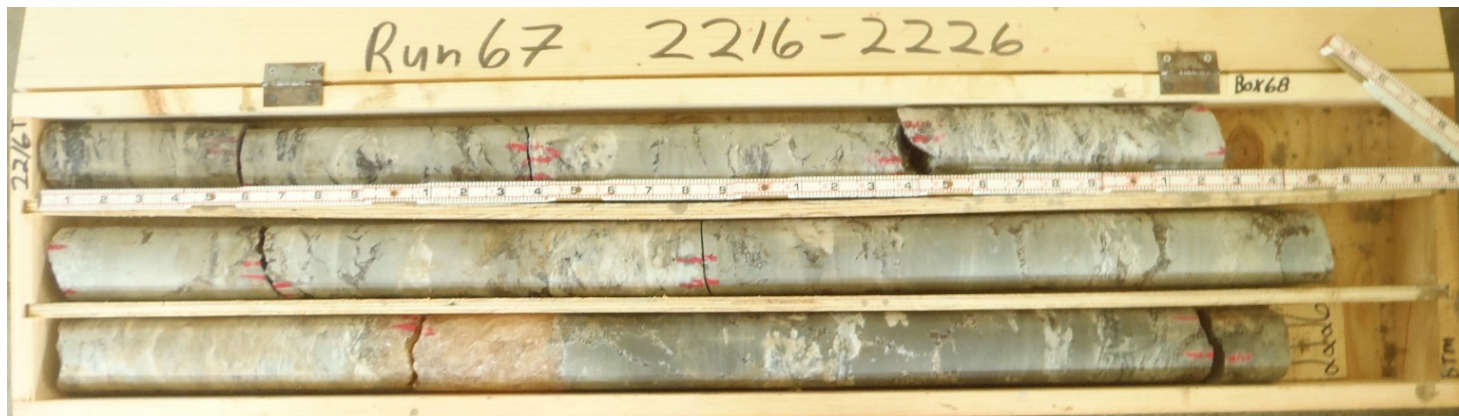
Figure B-78. Run 67: 2,216–2,226 Feet Below Ground Surface. Salina Group: Syracuse Formation–Salina E Member.
