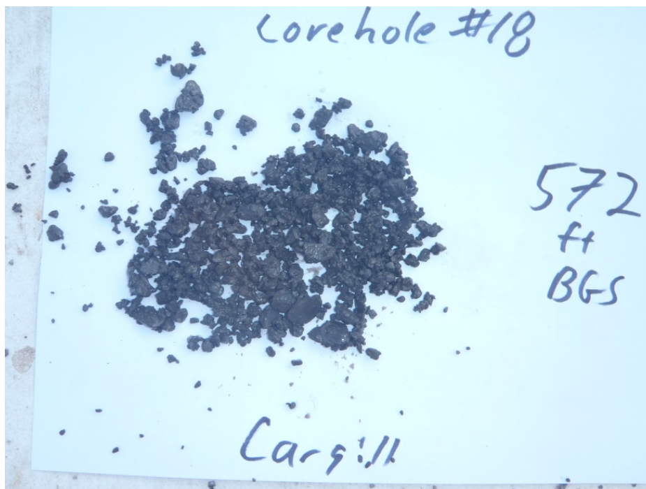
Figure A-29. Corehole #18: 572 Feet Below Ground Surface. Hamilton Group: Ludlowville Shale Formation–Ivy Point Member.
