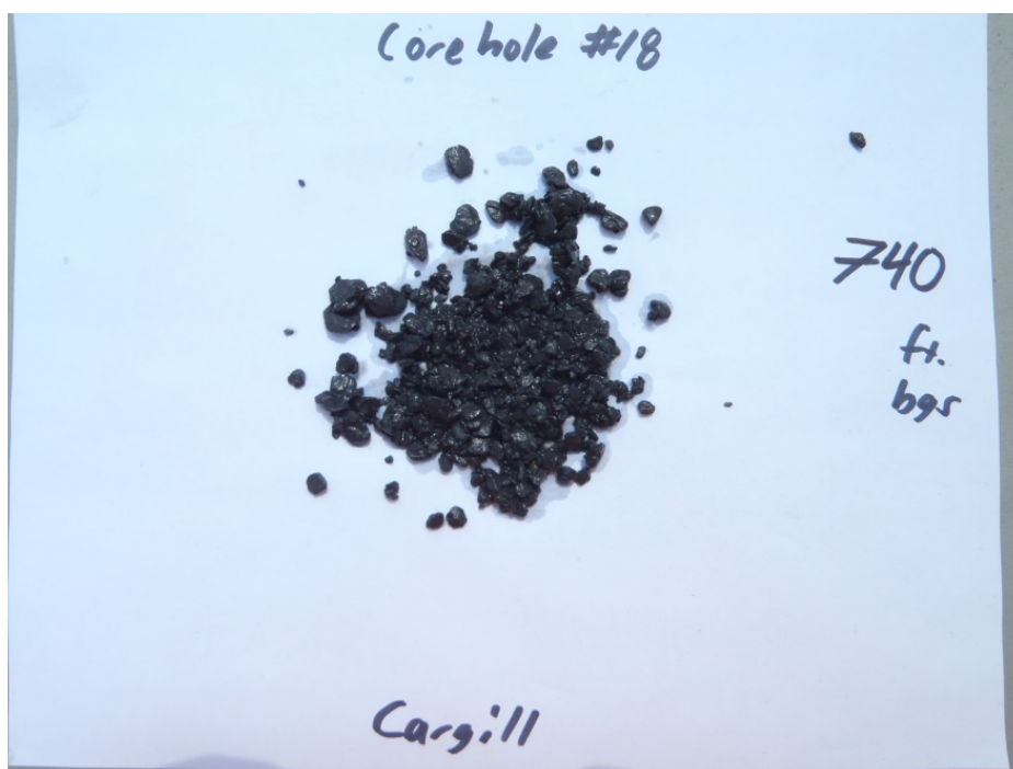
Figure A-38. Corehole #18: 740 Feet Below Ground Surface. Hamilton Group: Ludlowville Shale Formation–Otisco Member.
