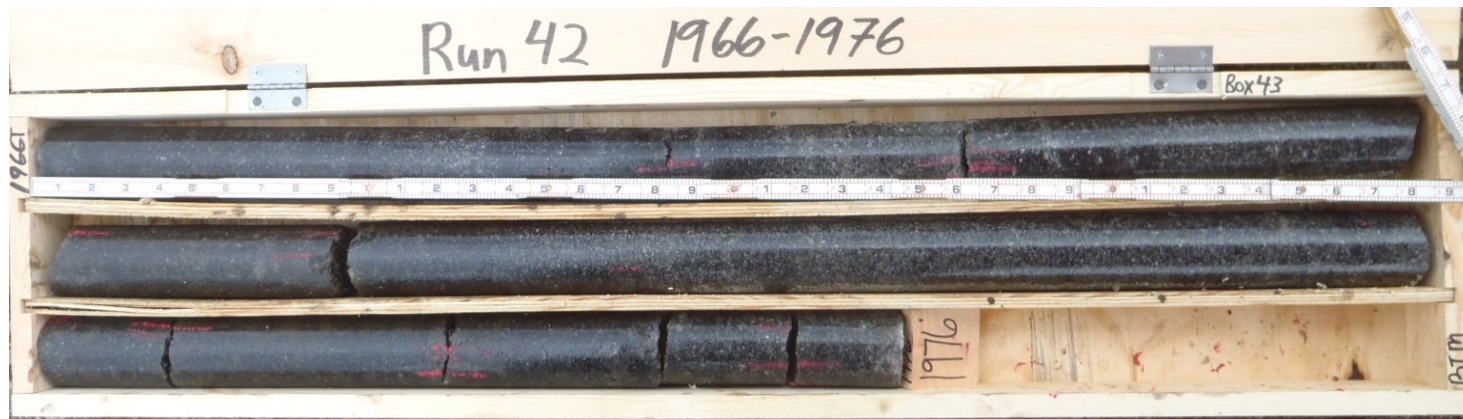
Figure B-49. Run 42: 1,966–1,976 Feet Below Ground Surface. Salina Group: Syracuse Formation–Salina F3/ #2 Salt.
