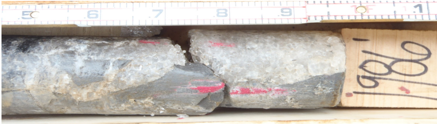
Figure B-51. Transition Zone at 1,985.6 Feet Below Ground Surface.
