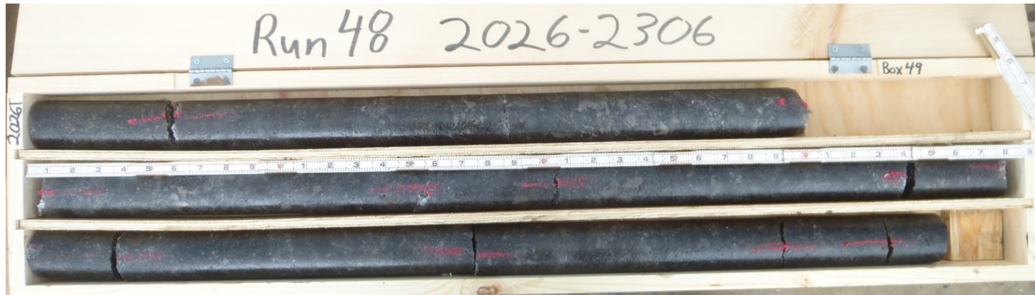
Figure B-59. Run 48: 2,026–2,036 Feet Below Ground Surface. Salina Group: Syracuse Formation–Salina F2/#3Salt.
