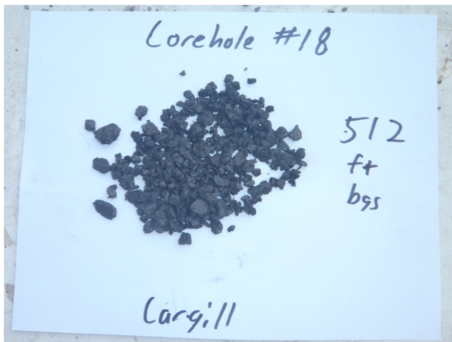
Figure A-26. Corehole #18: 512 Feet Below Ground Surface. Hamilton Group: Ludlowville Shale Formation–Spafford Member.
