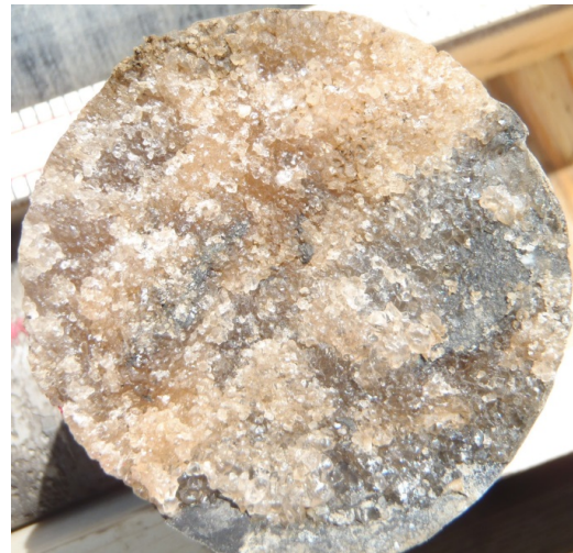
Figure B-37. Run 33: 1,876–1,886 Feet Below Ground Surface. Salina Group: Salina G/ Camillus and Syracuse Formation–Salina F Contact.
