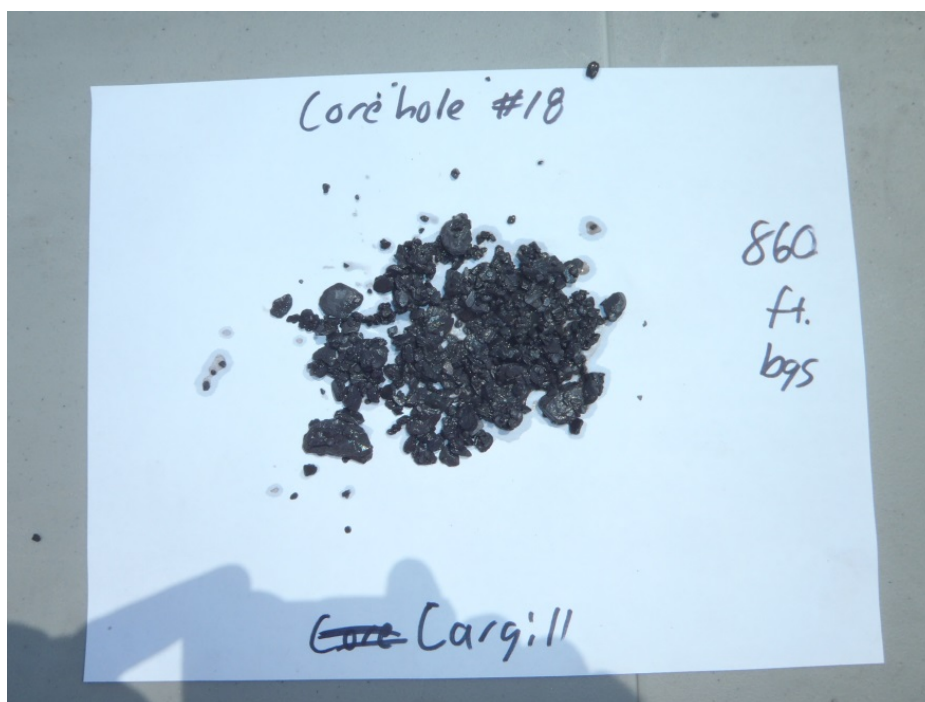
Figure A-44. Corehole #18: 860 Feet Below Ground Surface. Hamilton Group: Skaneateles Shale Formation–Butternut Shale Member.
